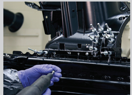
Can be weld bonded or rivet bonded within working time.
